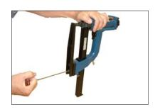
When *Anvil(029)* is properly aligned, tighten pivot *Screw(521)* first, then tighten retaining *Screw(514)*.
