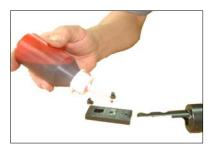
Reassemble New Driver Guide (016) and *Screws*(520).
