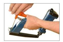
Align *Anvil*(029) with staple points by turning *Screw*(506).
